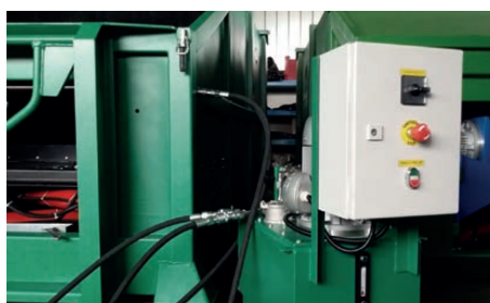
DEMONTIRAJUĆI AGREGAT SA KOMANDAMA DETACHABLE AGGREGATE WITH ALLOCATED COMMANDS
