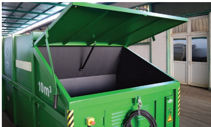
PRIHVATNA KOMORA / RECEIVING CHAMBER
