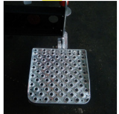
Amortizirani nogostupi za vožnju radnika-poslužioaca Amortized sidewalks for operator to stay during vehicle movement
