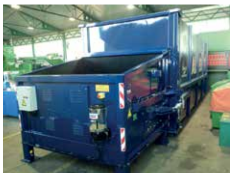
PRIHVATNA KOMORA RECEIVING CHAMBER
