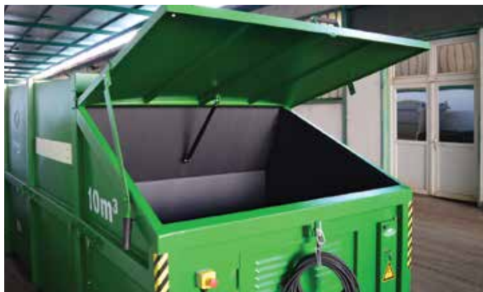
PRIHVATNA KOMORA RECEIVING CHAMBER
